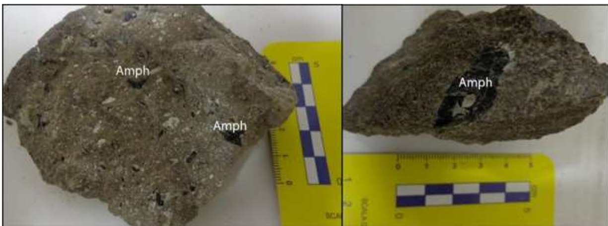
Figure 40 – Samples of alkali olivine basalt with amphibole megacrysts from Hoover Dam, Arizona.
