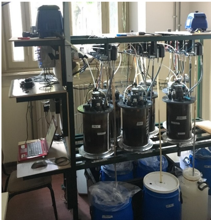
Figure 35 Schematization of the reactor and its components (a); functioning system of six reactors (b) operating with 3 different inlets.
