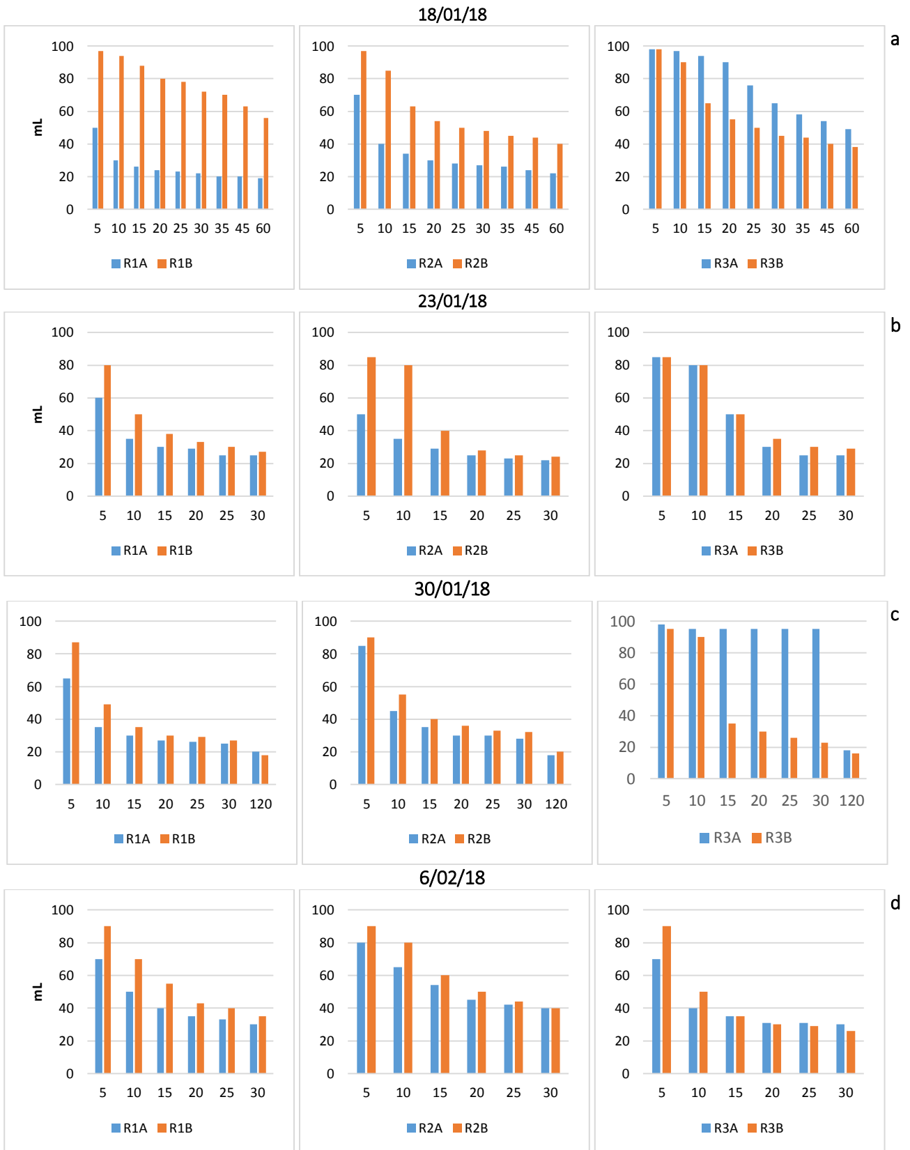
Figure 52 The performance of the activated sludge-water interface during the time for each pair of reactors on different days: a) 18/12/2018, b) 23/01/2018, c) 30/01/2018, d) 06/02/2012.
