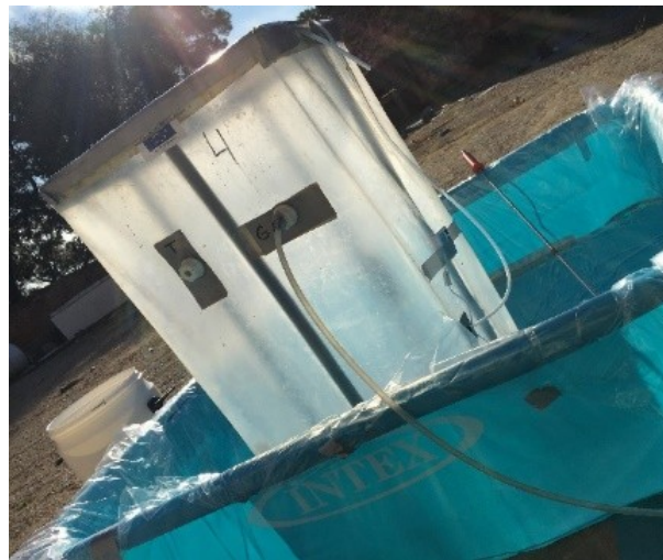
Figure 56 Two holes in the static hood (SH) used for withdrawing air sample and for measuring temperature inside the hood.
