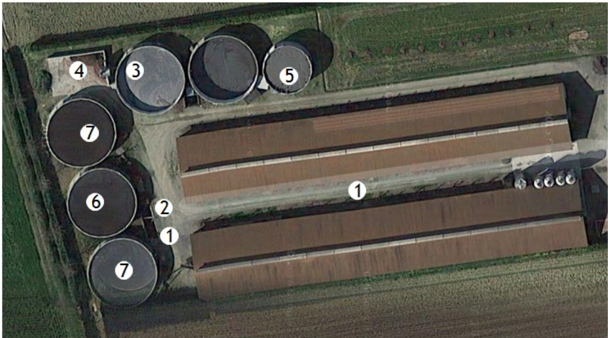
Figure 20 The overview of the plant VA. 1: inlet points; 2: tank for preliminary storage; 3: liquid fraction after solid/liquid separation; 4: solid fraction; 5 SBR plant; 6,7,8: storage tanks.
