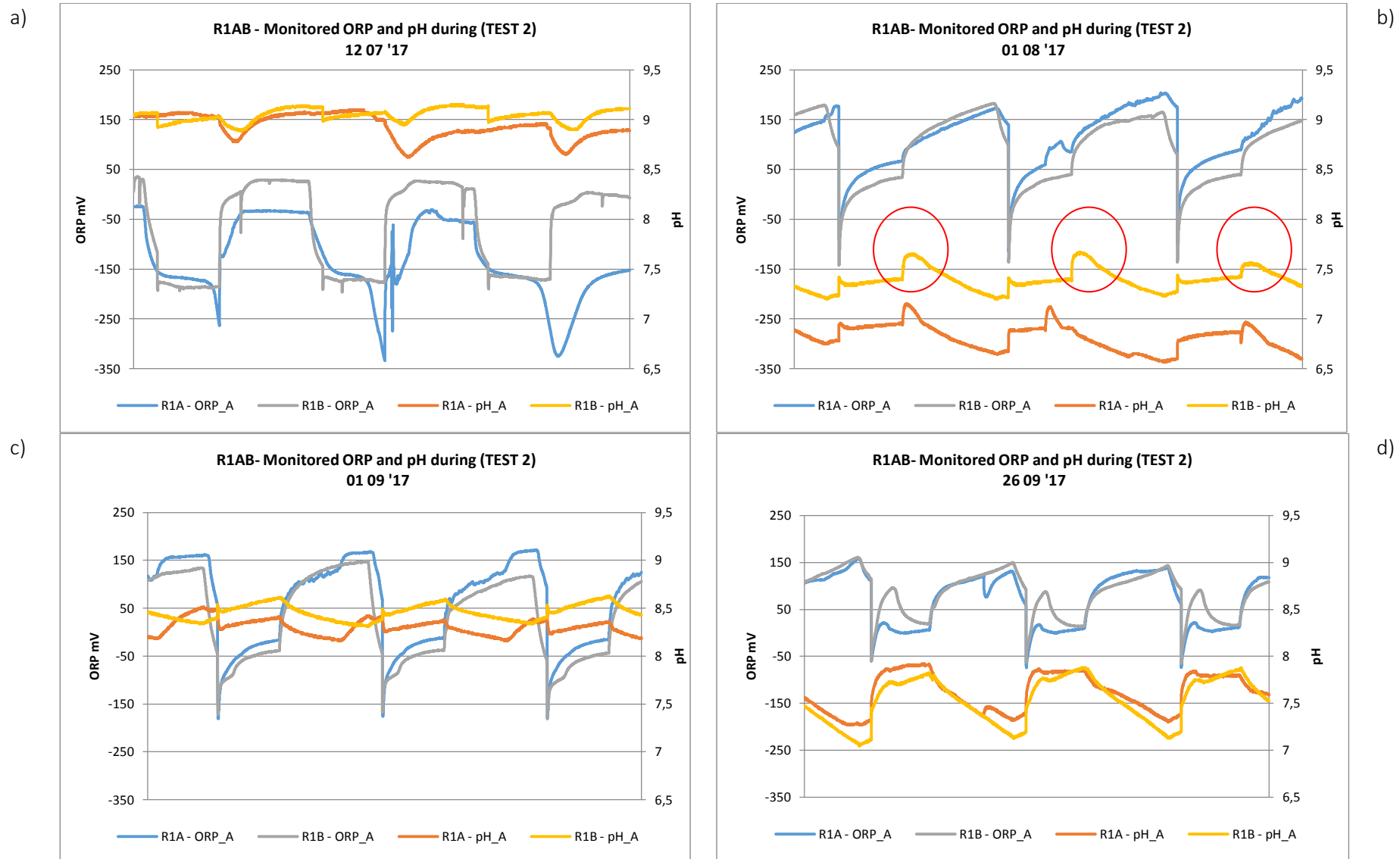
Figure 46 Trend of parameters monitored for reactors pair R1A e R1B during one day (24h), in particular: at the beginning of experiment (TEST 2), after about 1 month of operation, after about 2 and 3 months of operation.
