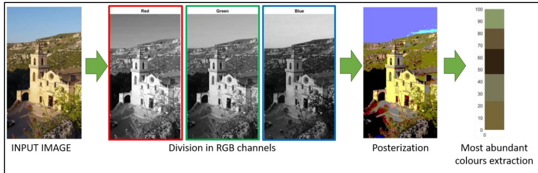
Figure 1 Workflow of the "Movie Barcode" algorithm.
