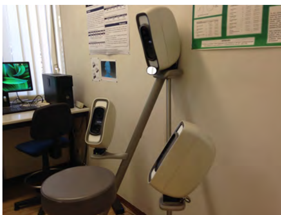
Figure 1. VECTRA M3 3D Imaging System (Canfield Scientific, Fairfield, NJ, USA): the three pods that surround the subject can be seen.
