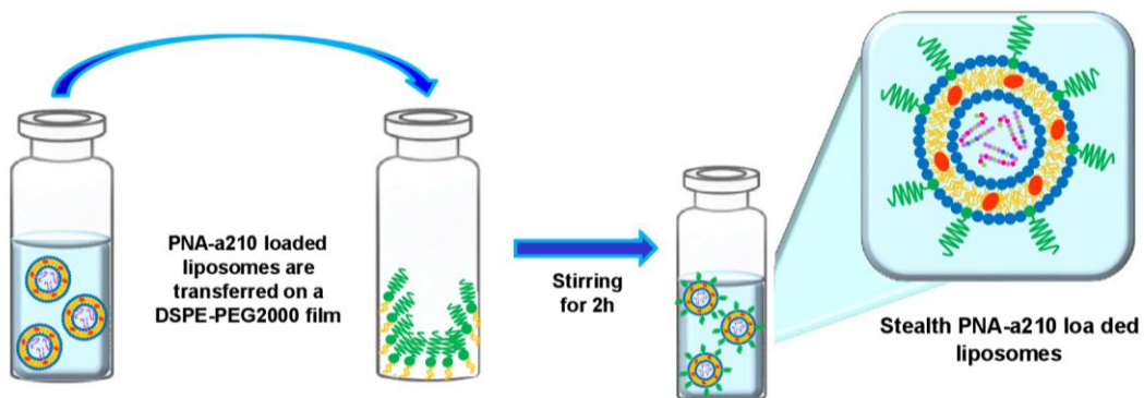
Fig.2. Preparation of PNA loaded liposomes in three steps: 1) the mixture of lipids was dried under vacuum to form a lipid film on the wall of the vial, then the film was hydrated and sonicated with the buffer; 2) PNA solution is added to the vial and liposomes undergone to five freeze/thawing cycles; 3) liposomes were made stealth by adding DSPE-PEG2000 using the post-insertion method.
