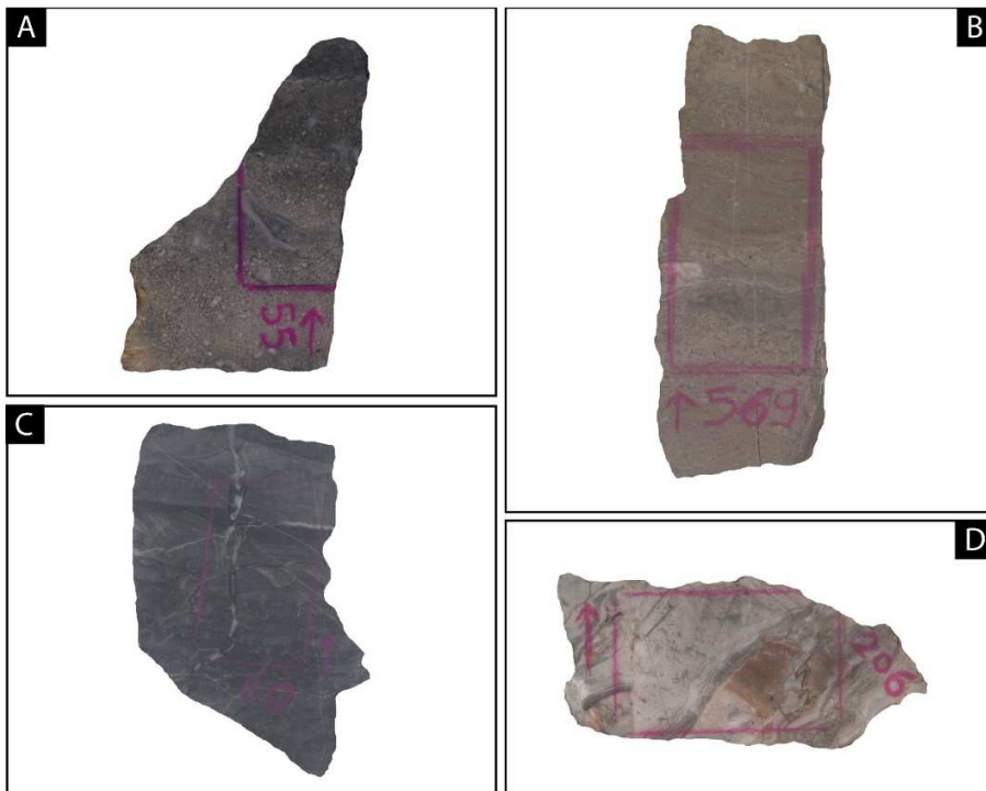
Fig.39 – Cut sample surfaces from Peritidal Esino Limestone. A) Sample TX55. Very coarse grained calcarenite (oid-oncoid grainstone). Coarsening upward pockets are visible. Piazza Brembana stratigraphic section (PB1). B) Sample TX569. Mid-grained calcarenite (peloid packstone and intraclast packstone) and microbial boundstone with fenestral cavities. Mt. Menna stratigraphic section (MNI). Microfacies in fig.40, B. C) Sample TX60. Black cement layer made of radial fibrous calcite. Piazza Brembana stratigraphic section (PB1). D) Sample TX206. Peritidal limestone breccia. Pink-reddish clasts are weathered limestone (intraclast packstone). Dark layers are microbial-cement coatings. The light grey part is a fine grained limestone (peloid packstone and clotted peloidal micrite) with fenestrae. Passo del Re stratigraphic section (PR1). The pink rectangle is 48 mm x 29 mm.
