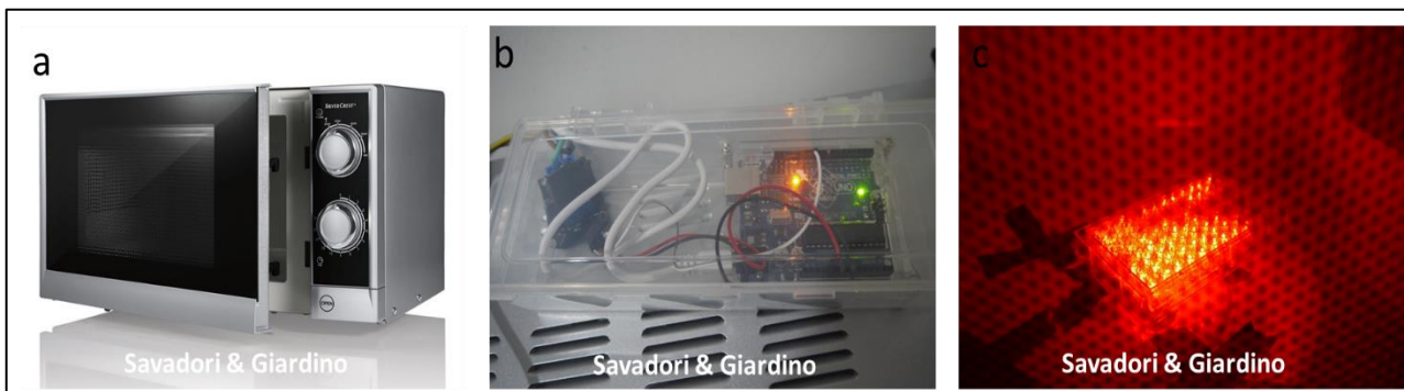
Fig 7: a) model of microwave used for decalcification procedure; b) Arduino board and relay; c) neon lamps array for the detection of cold/hot spots
