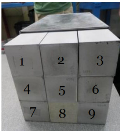
Figure 4.10: The first PARIS cluster. The detectors position numbers are marked. Taken from [84].
