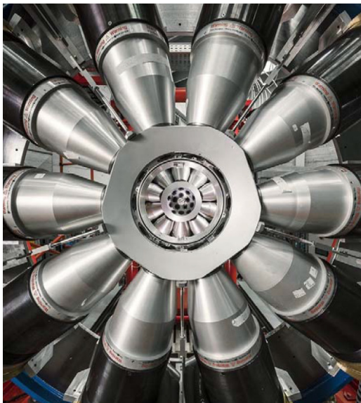
Figure 6.5: A GALILEO array (25 HPGe) picture taken from the beam dump. The central ring, with the 10 HPGe detectors, is visible, and it hides the 15 other detectors. Taken from [126].
