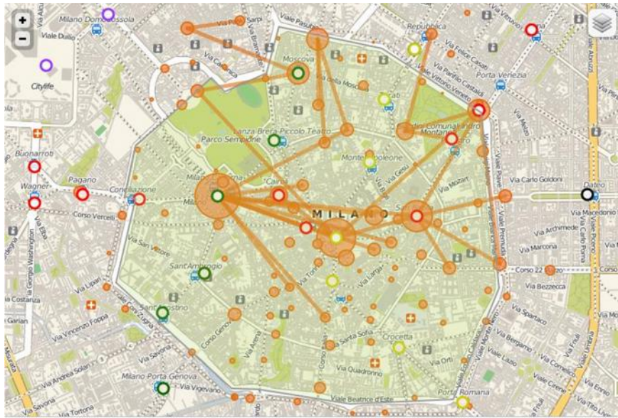
Figure 7 - Main cycling paths (highlighted in orange). The radius of the orange circles around the stations are proportional to the total number of trips. Other circles in red, light green and dark green represent Milan's underground stations. The light green area is the congestion charge area (Source: 2012, Clear Channel dataset and pedalami.it website)
