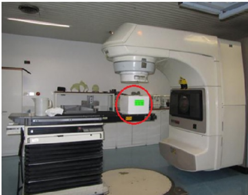
Figure 5.2: Photon beam irradiation setting: Varian 2100C linear accelerator at the Fondazione IRCCS Istituto Nazionale dei Tumori, Milano. The red circle points out the water phantom in which the flasks are placed.
