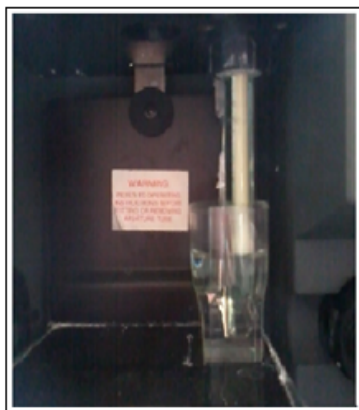
Figure 5.7: Beckmann Coulter Counter. The tube is immersed in the glass containing the isotonic solution with cells to be counted.
