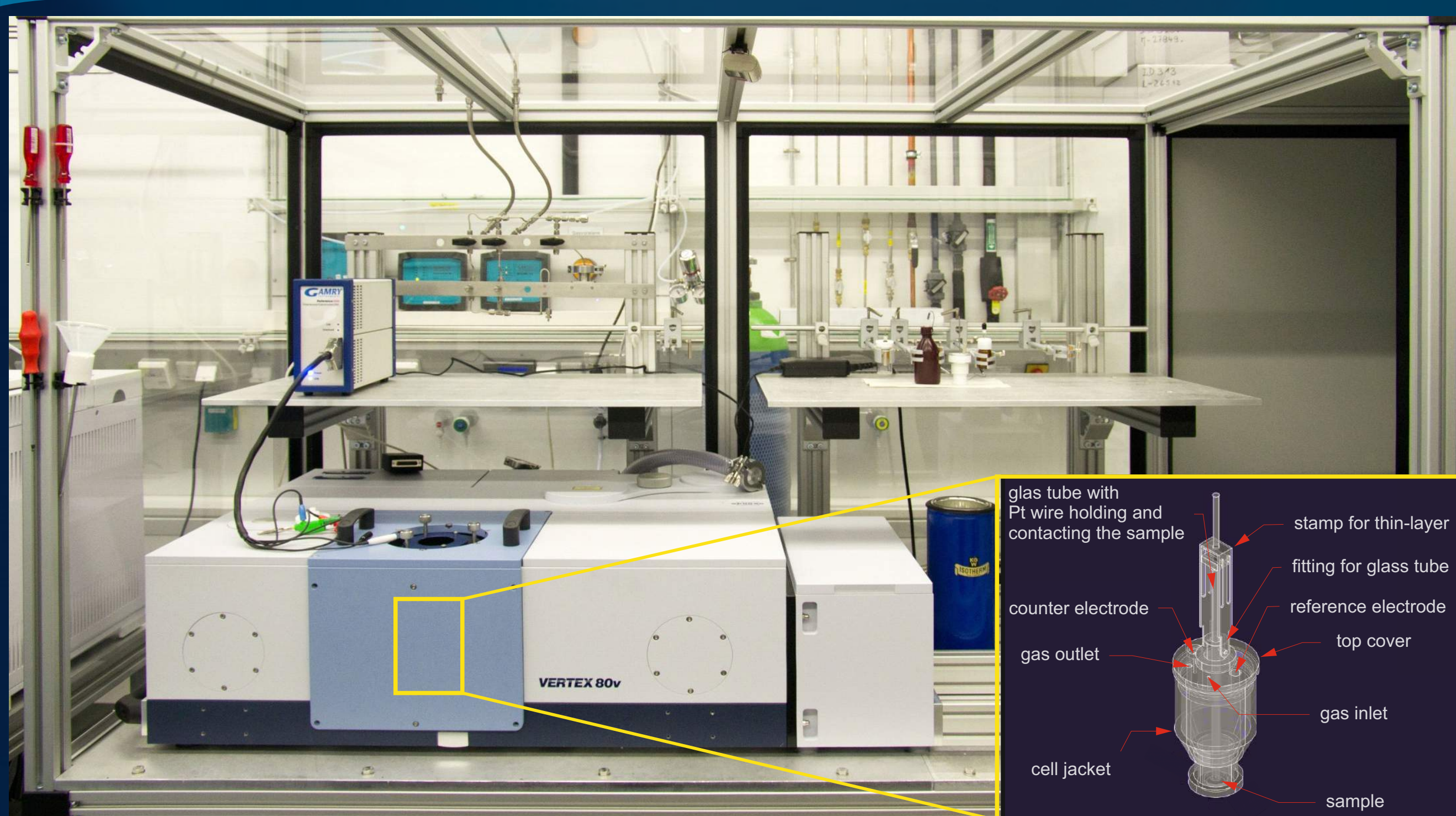
IR spectro-electrochemistry including vacuum FTIR spectrometer (Bruker Vertex 80v), gas inlet system, and new home build external reflection cell.
