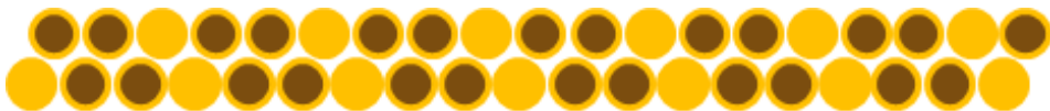
Figure 4.6: Alternative option for the low field cable . Superconducting strands are represented as brown circles with a yellow jacket, pure copper strands are represented as yellow circles
