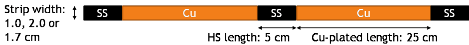
Figure 4.21: A heater strip geometry: Each strip has 5 cm long stainless steel heating stations placed with 30 cm period. Three different strip widths are used: 1.0, 1.7 and 2.0 cm.
