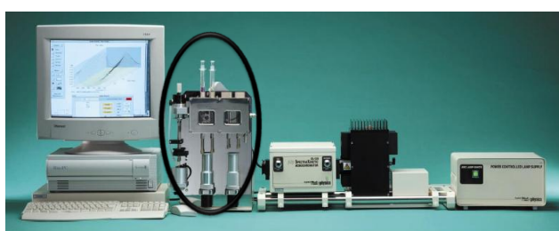
Figure 2.1: The stopped-flow instrument and its diagrammatic representation.
