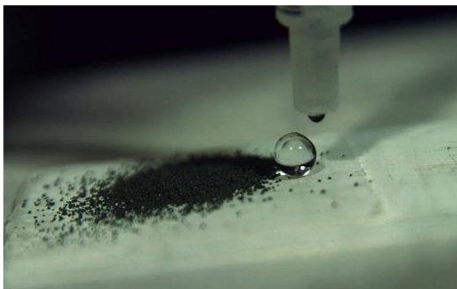
Figure 26. Dripping water on SPES_I.Ls. during self-cleaning test.
