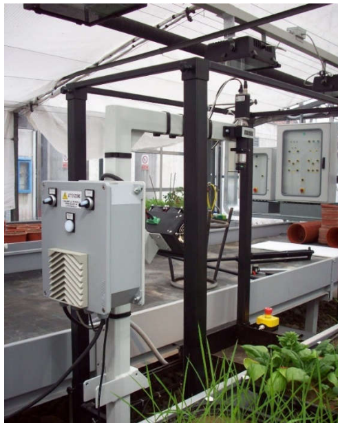
Figure 1. – Image of the sliding platform and of the hyperspectral imaging sensor in the greenhouse.
