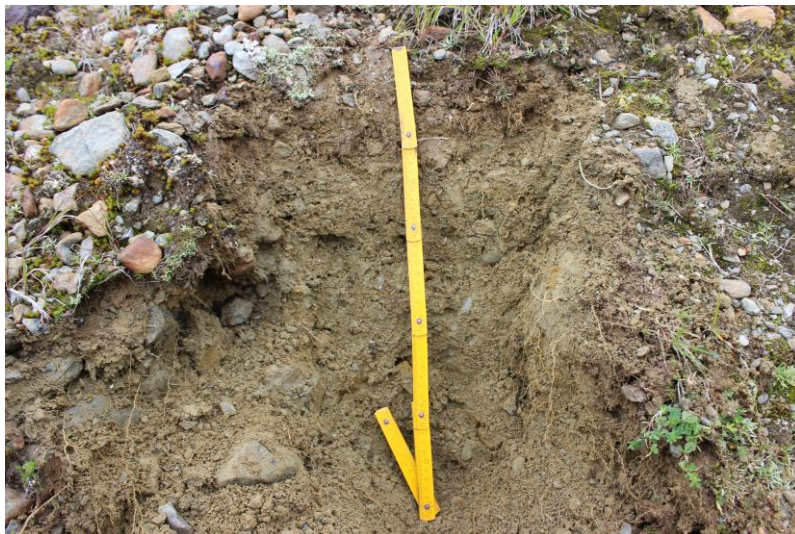
Figure 7. The soil properties of profiles detected in a plot are investigated. In the image, the identification of the horizons and their depth are being performed (photos: F. Sobacchi; summer 2014).
