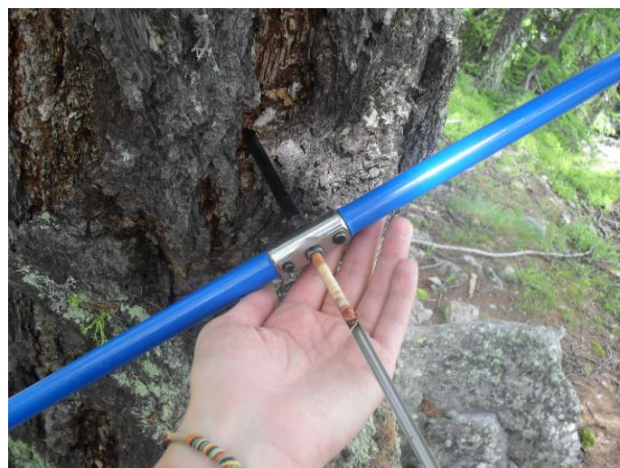
Figure 9. Tree sampling using a Pressler's increment borer.
