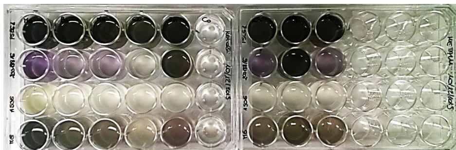
Figure 2.6: Effect of the single micronutrients on the blue pigment production. Test on strains UMB248, UMB258 and 200188/6 are shown. Metals order: Mo, Bo, Mn, Cu, Zn, Co, Ca, Mg, Fe.
