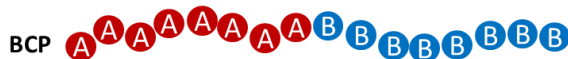
Figure 1.2: Example of a diblock copolymer chain displaying two different blocks of the monomeric components A, B.
