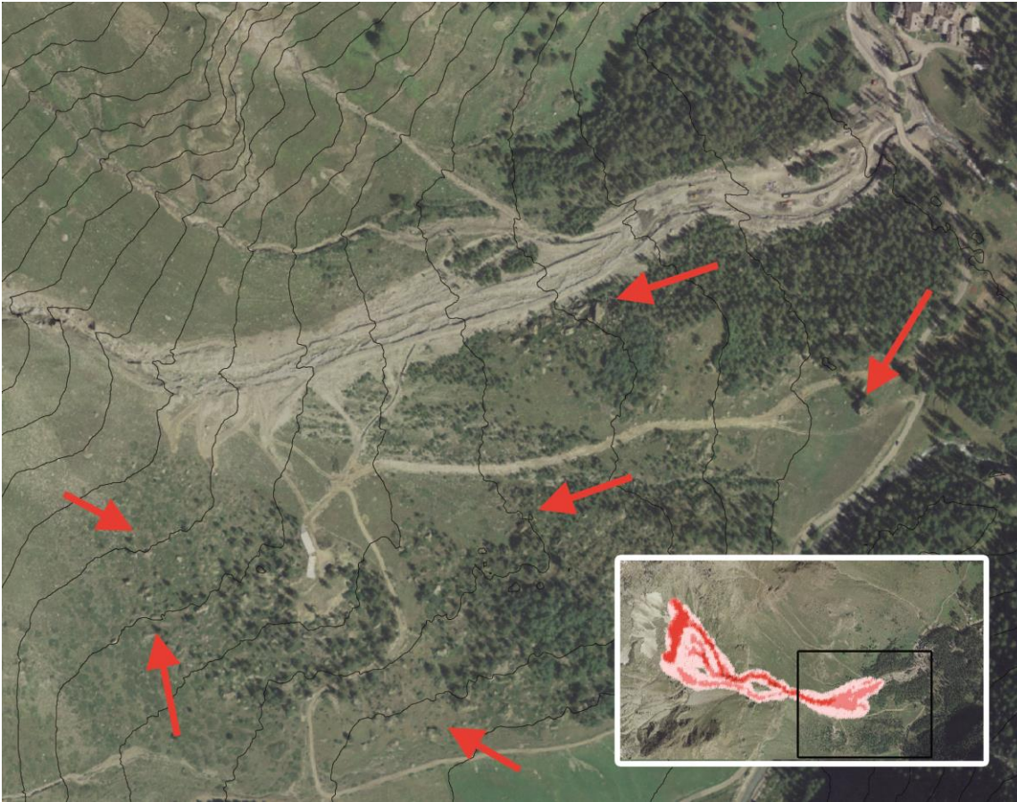
Fig. 12 Details of the Pellaud channel. Arrows indicate the presence of rock blocks deposited during past events. The contour interval is 20 m.
