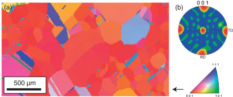
Figure 4.2: (a) Electron back scattering diffraction map acquired on a graphene grown on Cu foil sample. (b) Orientation distribution of the image reported in (a). The dominant crystalline orientation is (001).
