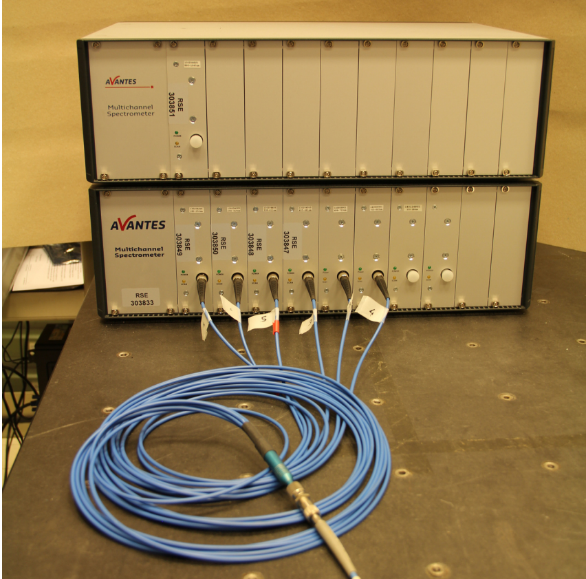
Figure 3.5 – A picture of the spectrometers with the optical fibers.
