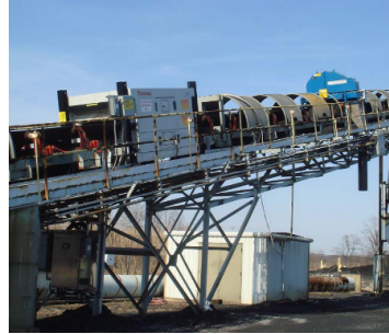
Figure 1.3 – Pictures of two online PGNAA element analyzers. Courtesy of DFMC Ltd. and Thermo Fisher Scientific Inc.
