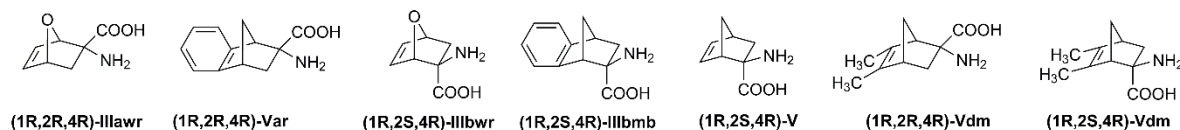
Figure 6.8. Structurally modified cCTAAs used for the study of mechanisms of helical screw sense preferences.
