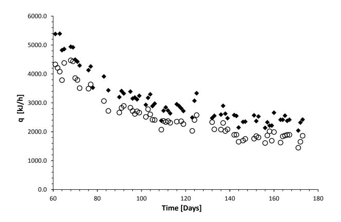
Figure 7 Absolute value of the heat transferred vs time.  $\blacklozenge$  Coated heat exchanger;  $\circ$  Uncoated heat exchanger.
