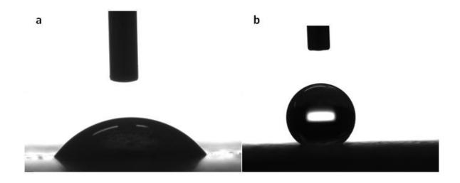
Figure 2 Contact angle measurements photos. Liquid droplet of distilled water deposited on (a) uncoated stainless steel surface and (b) coated stainless steel surface.
