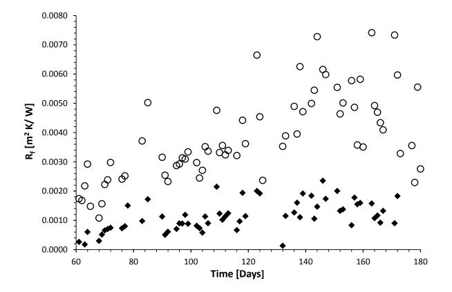
Figure 6 Fouling resistance *vs* time. ◆ Coated heat exchange ○ Uncoated heat exchanger.
