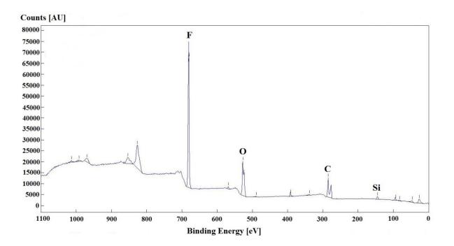
Figure 3 XPS survey analysis in the whole range of X-ray spectrum. Composition table: Si = 3.6 % at; C = 31.4 % at; O = 23.5 % at; F = 41.6 % at.
