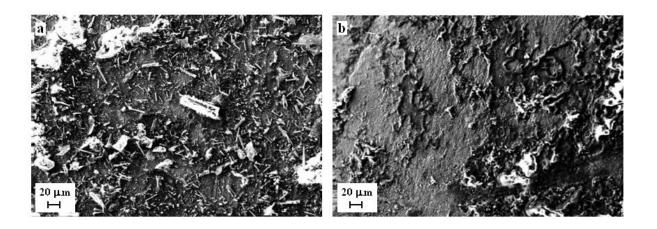
Figure 8 SEM images of fouling deposits formed on the internal tube surface of the (a) coated heat exchanger and (b) uncoated heat exchanger.
