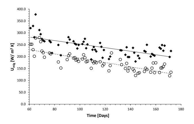
Figure 4 Overall heat transfer coefficient vs time.  $\blacklozenge$  Coated heat exchanger;  $\circ$  Uncoated heat exchanger.
