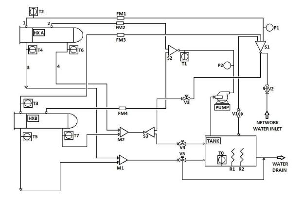
Figure 1 Flow sheet of the pilot plant. HX A: Heat Exchanger A; HX B Heat exchanger B; --1--Shell side inlet flows; --2-- Tube side inlet flows; --3-- Shell side outlet flows; --4-- Tube side outlet flows; V: valves; T: thermocouples; FM: flow controllers; S: splitter; M: mixer; P: manometers; R1/R2: heating units.
