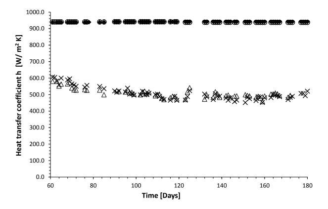
Figure 5 Comparison between shell-side and tube-side heat transfer coefficients of coated and uncoated heat exchangers.  $\blacklozenge$  h<sub>H</sub> for coated heat exchanger;  $\circ$  h<sub>H</sub> for uncoated heat exchanger;  $\triangle$  h<sub>C</sub> for coated heat exchanger;  $\times$  h<sub>C</sub> for uncoated heat exchanger
