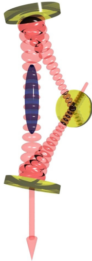
Figure 1.5: Schematic representation of a three-mirror ring cavity designed for continuous detection of Bloch oscillations of atoms falling inside a vertical light wave sustained by the cavity.
