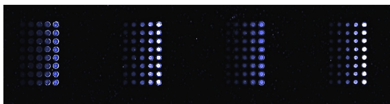
Figure 4.17: Aptamer-microarray - Microscope slide coated with a thin film of nano-structured zirconia with spots of aptamers (described in table 3.2).
