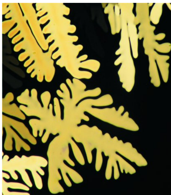
Figure A.9 - Dendritic growth of columnar C_2 phase in a sDNA 12TT sample. Photo by Michi Nakata.
