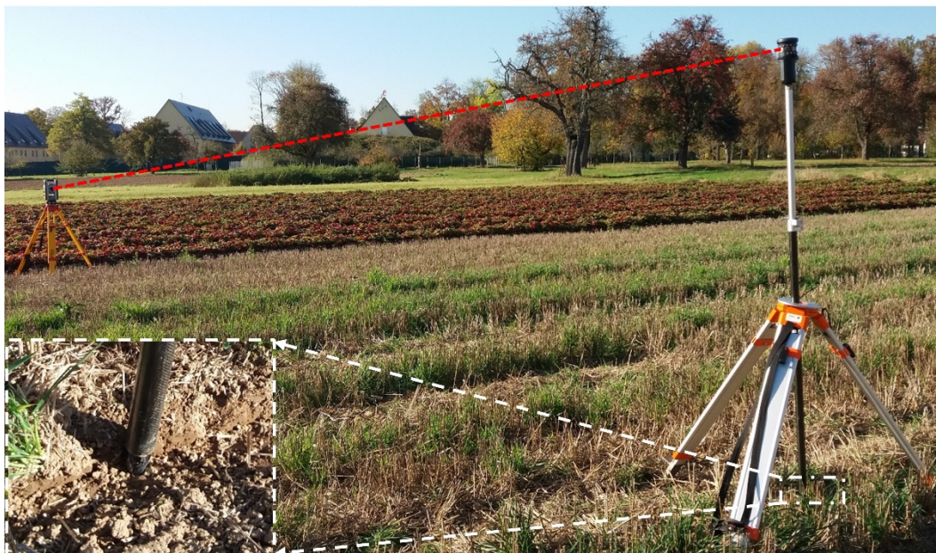
Figure 4.4. Measurement for geo-referenced seed positions.
