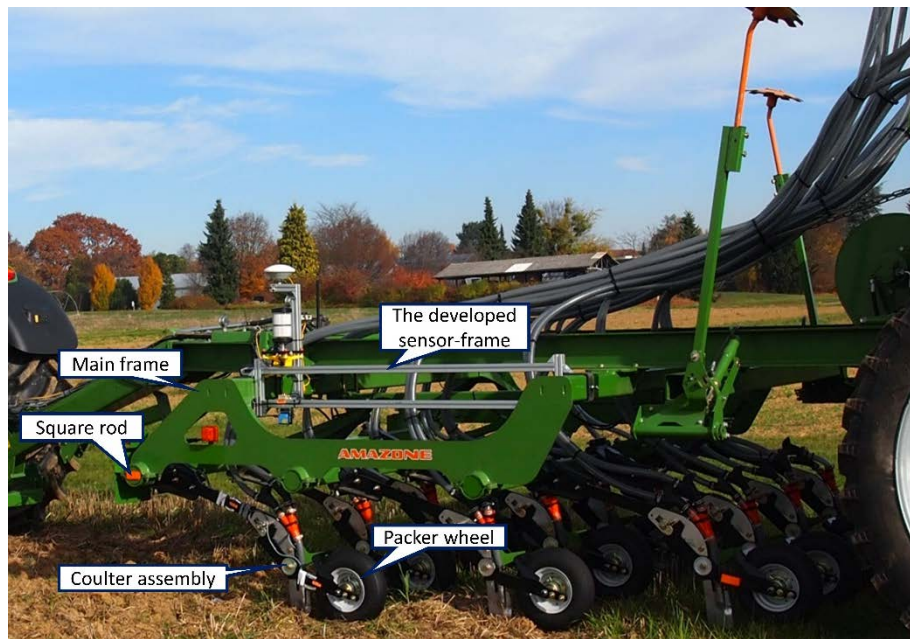
Figure 3.1. The configuration of the utilised no-till direct seeder.
