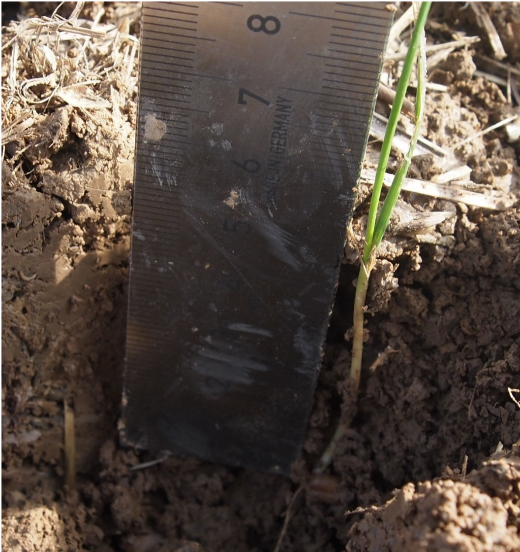
Figure 2.5. The ground truth seeding depth measurement from seedlings.
