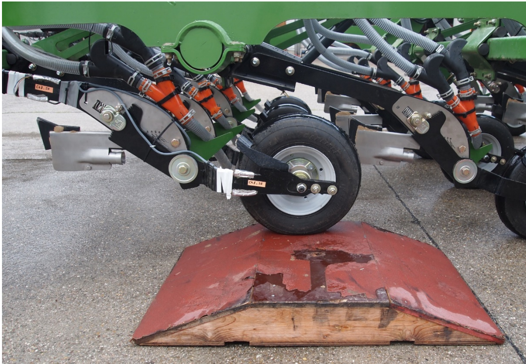
Figure 2.2. Measuring the profile of a trapezoidal bump.
