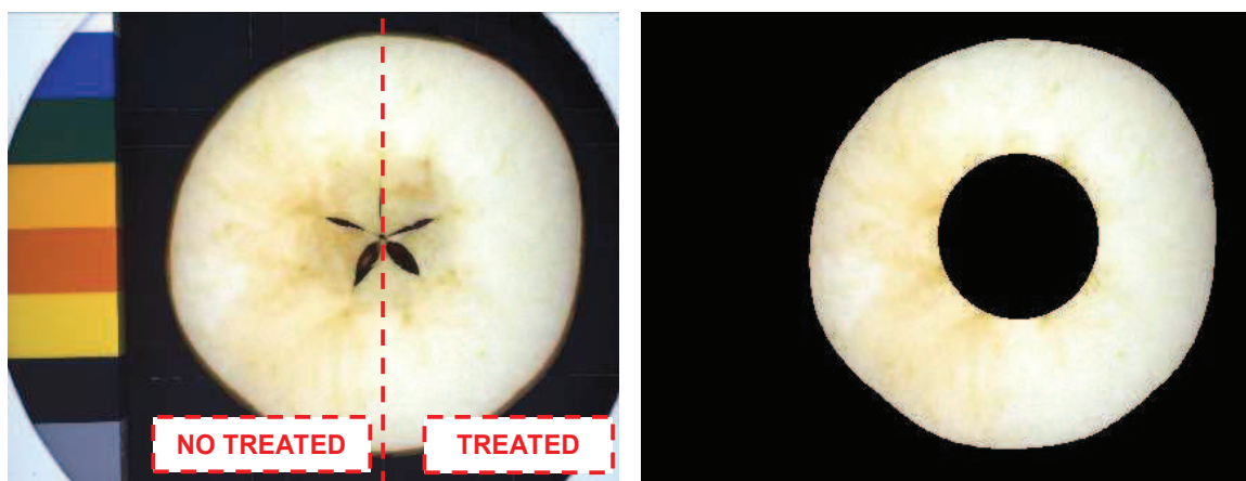
Figure 1. RGB picture of an apple slice (on the left) with labels indicating the L-ascorbic acid treatment. Furthermore, all the visible regions are visible: the apple slice (composed of the flesh, the core and the peel), the multicolored reference, the background and the integrating sphere borders. Final identification of the region of interest (on the right), after the masking procedures.
