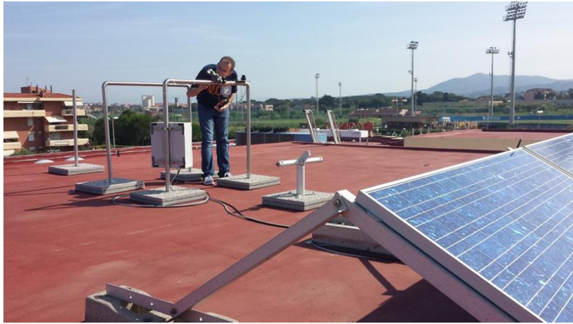
Figure 29: Photo during the installation of the solar measurement station at Flyby (Livorno, Italy). The Author is setting the position of one of the UV sensors.
