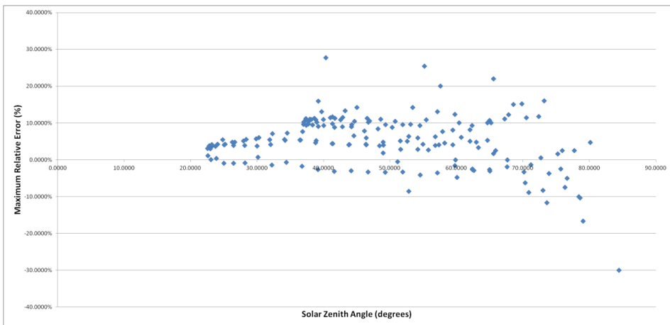
Figure 63: Maximum relative difference between satellite-based and in-situ measured UV dose data with respect to SZA in stable weather conditions. Data are referred to the Saint Christophe (Aosta, Italy) station in the period June-July 2014. Taken from (Morelli, Masini and Diémoz, et al. 2014).
