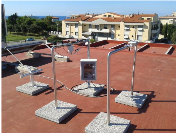
Figure 39: Photo of the solar radiation measurements station and the horizon seen from the roof of Flyby (Livorno, Italy) on September 6 th 2014.
