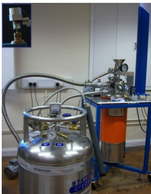
Figure 3.6: Resonant ultrasound spectroscopy apparatus used for the elastic measurements. The inset at the top-left corner shows the head where the sample is located.
