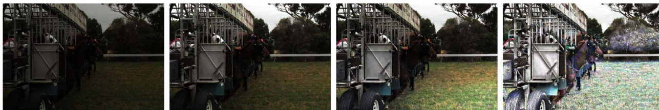
Fig. 7. Comparison among results with different a values [see Eq. (6) and same percentile (99th)]. The first image is the original; then a = 1, 2, 3 .
