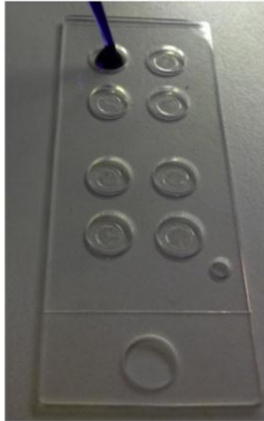
Figure 5.4 - Picture of the multiwell system used to compartmentalize eight hydrogel plugs. The hydrogels are made of a DMA-Bis solution (4% T, 3% C) that can be desiccated and rehydrated in 60 min by adding 30 \mu L of desired solution [Sola et al., 2013].
