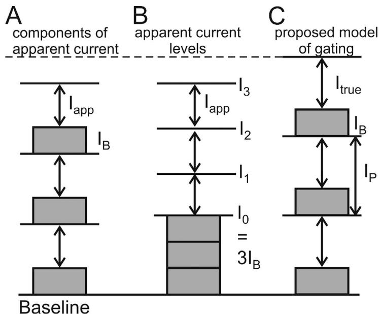
**Figure 1.** Definitions of current components used in data analysis. (A) Contribution of the constant ( $I_B$ ) and flickering components ( $I_{app}$ ) of each pore to the measured single-pore current. (B) Illustration of the levels  $I_0$  to  $I_3$  observable in a measured time series. (C) Scenario used for fitting amplitude histograms.  $I_p$  is the sum of  $I_B$  and the true (reconstructed by fitting) single-pore current  $I_{true}$ .
