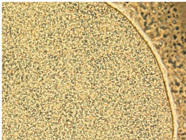
Figure 5.19: Phase contrast image of granular phase of sticky-end 5'-GCTA-3', considerable difference in refractive index between grains and background is evident.
