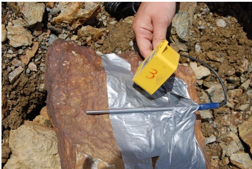
Fig. 3: The thermistor (Tinytag) installed at the base (bottom face) of a flat (ca. 2 cm deep) rock following the protocol of the permafrost (see Osterkamp, 2003; Guglielmin, 2006; Guglielmin et al., 2008).
