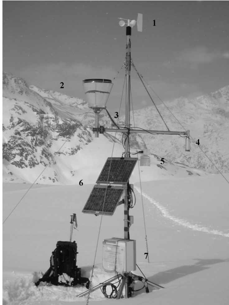
Fig. 2: AWS1 Forni. The instruments are marked with numbers: (1) wind speed and direction, (2) rain gauge, (3) net radiometer CNRI, (4) sonic ranger, (5) thermo-hygrometer, (6) solar panels, and (7) barometer inside the datalogger box (photo by G. Diolaiuti).
