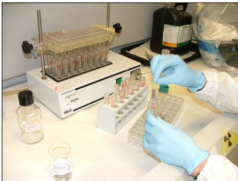
Figure 12: trimmed hair are added with 3 ml of methanol and incubated at 37°C for 18 hours (photo: C. Caslini).
