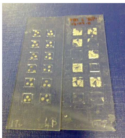
Figure 10. Hydrogel plugs with good adhesion (left, DMA 4% - BisA 3%) and bad adhesion (right, DMA 8% - bisA 5%) to the ITO surface.
