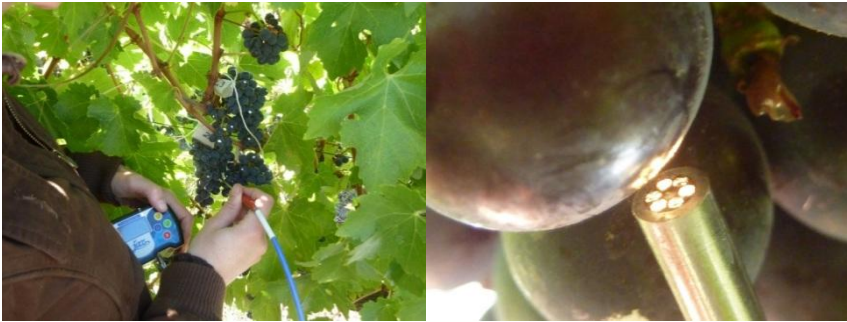
Figure 1. Images of spectral acquisition phases on fresh berries with the JAZ system
