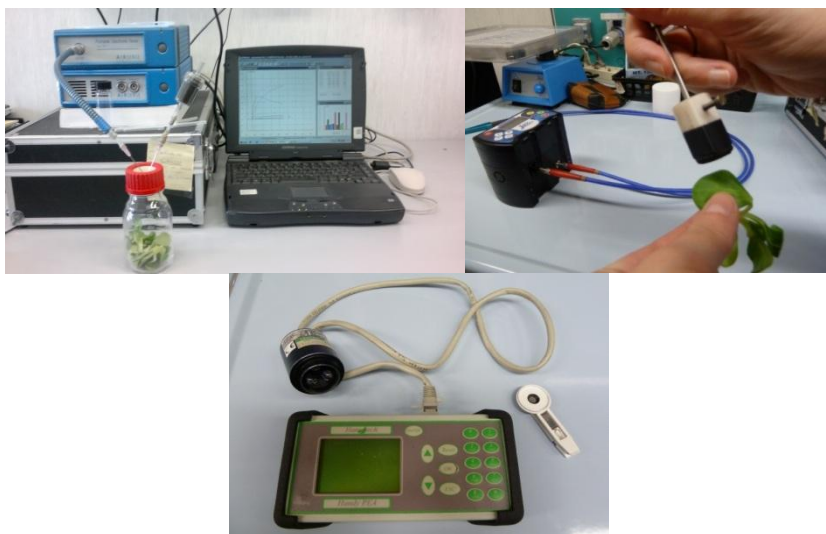
Figure 1. From left to right: Electronic Nose (PEN 2, Win Muster Airsense Analytics Inc., Germany); JAZ vis/NIR spectrophotometer, OceanOptics, USA; Handy Plant Efficiency Analyser (PEA, Hansatech, UK)
