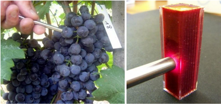
Figure 9. Images of spectral acquisition phases on fresh berries and on homogenized samples.
