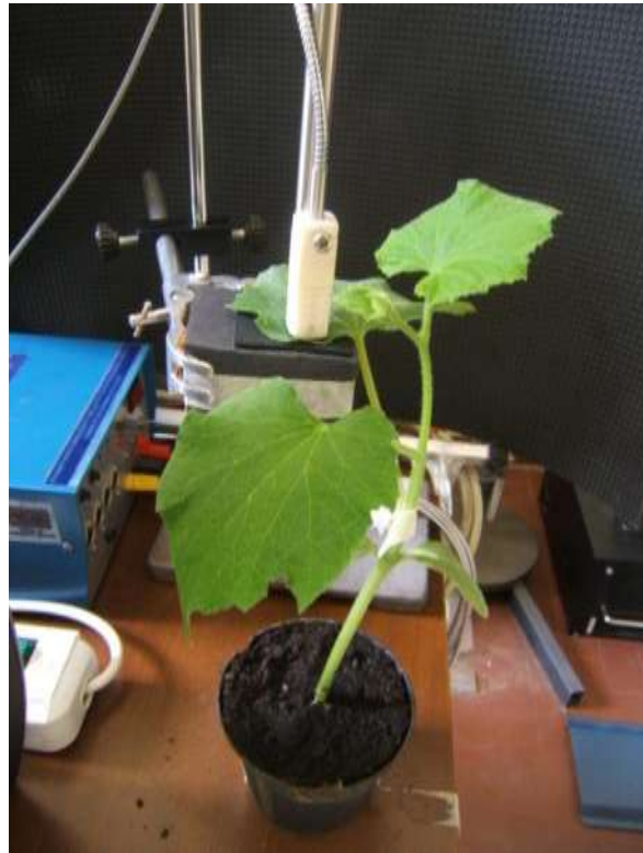
Figure 29 - Experimental setup: measures of reflectance. You can the analysis station consists of a support of black color (black box) provided with a soft surface on which to lay carefully the leaf. The measurement is achieved by the use of an optical fiber that channels the light emitted by the LED. At the end of the optical fiber which emits the light radiation (and channels the radiation reflected by the leaf surface) is present a white box used as a darkroom.
