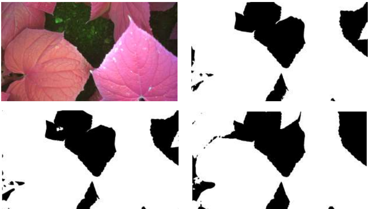
Figure 66 – Example of test image using the topsoil as a background where more plants are acquired by multispectral camera (upper left), its manually painted binary masks associated (upper right), the Background Removal algorithm result using the Expectation Maximization algorithm (bottom left) and the Background Removal algorithm result using the Otsu Threshold algorithm (bottom right).
