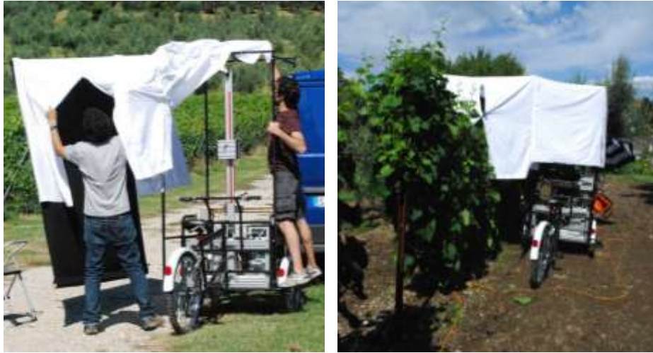
Figure 35 - Instrumented field trolley hosting the acquisition system. Canopy imaging is done inside a tunnel structure providing background regularization and diffuse illumination of the measured area.
