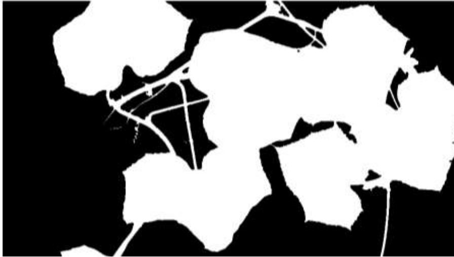
Figure 64 - Binary image resulting from thresholding of the image shown in Figure 60 with the threshold value (Figure 63) identified by the Background algorithm.
