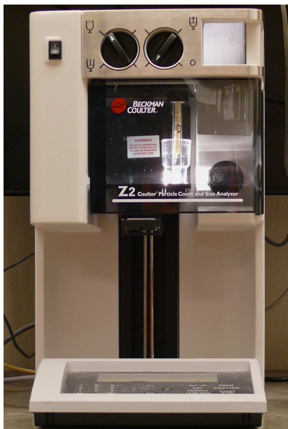
Figure 3.3. Determination of granulosa cell numbers using a Z2 Coulter® Particle Count and Size Analyzer.
