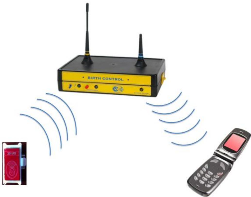
Figure 19: The transceiver is attached at vulva lips in pregnant cows and when it is activated by fetal membranes expulsion a radio wave signal is sent to a receiver-transmitter. Through the use of the Global System for Mobile communication (GSM) technology the receiver sends a short text message (SMS) to the farmer's mobile phone warning him of the coming delivery.
