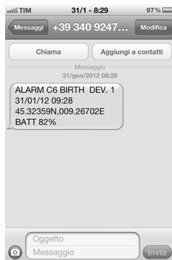
Figure 6: birth alarm message received on the breeder's mobile phone.
