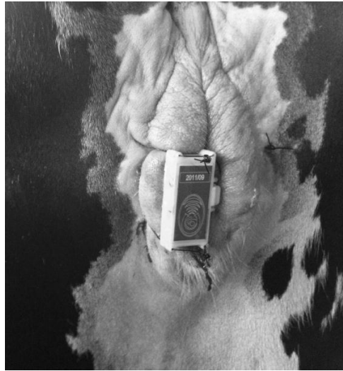
Figure 2: Close up of the vulvar sensor applied to a cow. Totally it can be seen 3 points suture for the fixing of the two parts of the sensor to the animal's big lips.
