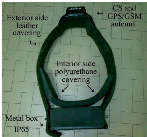
Figure 1. The GPS-ACT collar with the components
