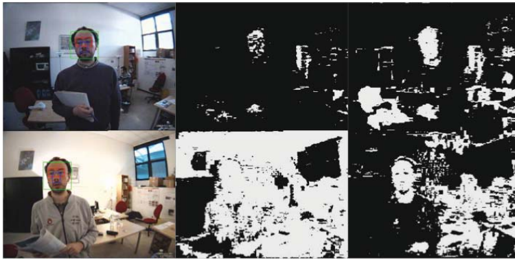
Fig. 1. Face and face features detection in different illumination conditions: natural lighting on the top row, neon lights on the bottom row. The centre and right columns show binary maps output of skin detection, with (right) and without (centre) white balancing.
