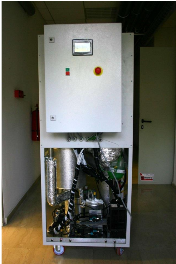
Fig. 2: Picture of the fuel processor (external FC unit not included). Size in cm: 70 x 100 x 180.
