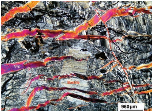
Figure 4. Orthopyroxene porphyroblasts replaced by bastite and crosscut by veins of serpentine; NX, 2X.
