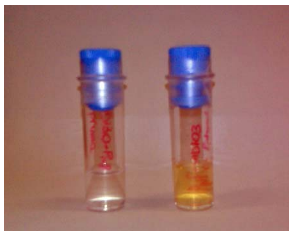
Figure 3. Water dispersion (0.1% v/v) of 1 -coated PnPs before (left) and after (right) photopolymerization promoted by 15 min exposure to 266 nm UV laser light.
