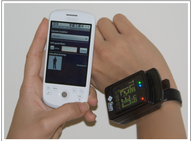
Fig. 7 The Android smart phone and Sun SPOT sensor used for the experiments
