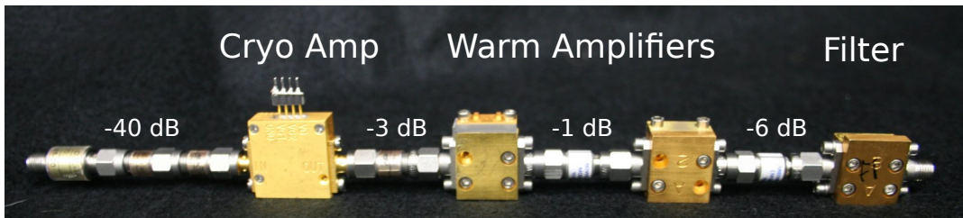
Figure 3. COFE 10 GHz radiometer VNA test setup for bandpass characterization
