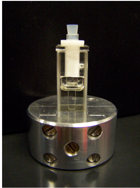
Figure 2.12: Sample cell for Dynamic Light Scattering measurements.
