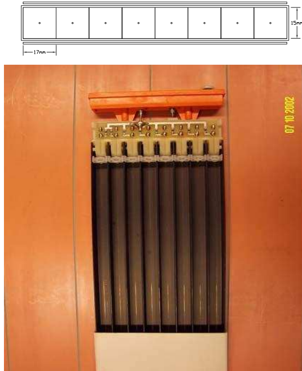
Figure 2.14: Sketch of an 8-cell module (top), and photo of an LST partially inserted in the sleeves (shown at the bottom of the picture).
