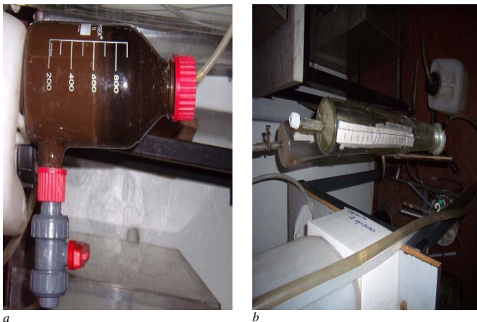
Fig. 1 – Experimental set up. a digester b column for biogas measurement
